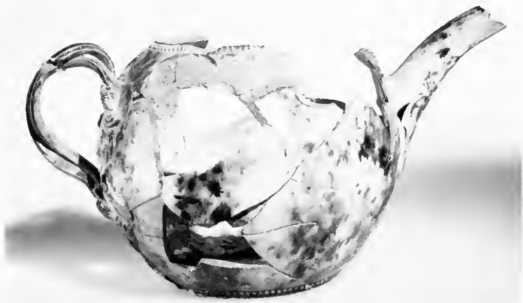
Figure 14. Creamware teapot with manganese mottling, Salem, North Carolina, 1770-85. This teapot was involved in a kiln accident, for spalling of the body underneath the rim is evident. Its mottled glaze is dark due to overfiring. HOA (through spout) 3 5/8"; WOA (body) 4 1/4". Courtesy of Old Salem, Inc. MRF S-1929.
